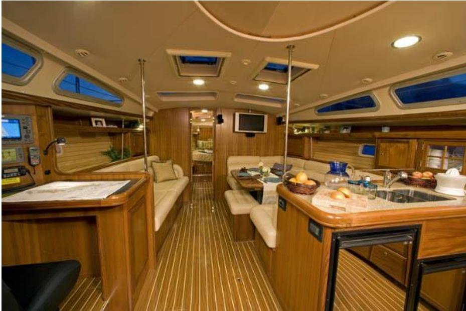
Numerous, handholds in the saloon (two study posts near the companionway and grab-rails below the ports) provide uninterrupted brace points for navigating around the large cabin. However, the grab-rails had a bit of give when I really yanked on them, and the companionway needs additional handholds so there's something to hang on to when you're on the first step. Whatever you do, don't grab the purely, ornamental light strip that's built into the vinyl headliner near the coachroof.
